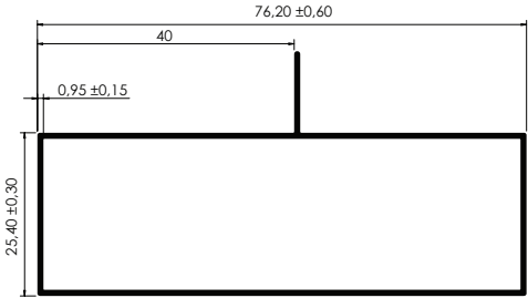
TUBO 3" x 1" CON ALETA 3" x 1" Hollow Tube with Fin
